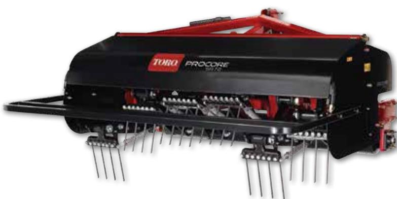
The ProCore SR Series provide working widths of 122 – 190 cm (48" – 75"), working depths up to 40.6 cm (16") and hole spacing from 6.3 – 15.2 cm (2.5" – 6").
